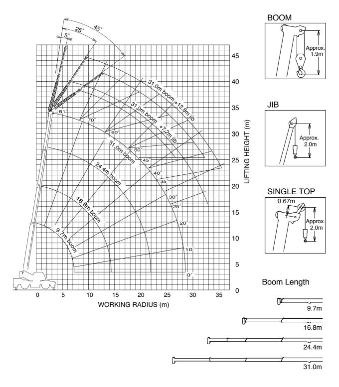
**NOTE:** The above lifting height and boom angle are based on a straight (unladen) boom, and allowance should be made for boom deflection obtained under laden conditions. The above working range is shown on condition with outriggers fully (6.3m) extended.
